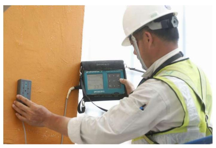
A tester deploying ultrasound scanning to check on all sunshades in Block 201E, Tampines Street 23, on Sept 30, 2016. ST PHOTO: CHEW SENG KIM
