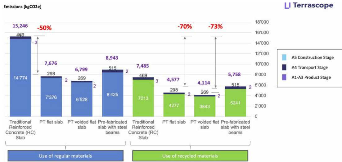
Comparing various CO2 Emissions of PT versus other construction methods (combined with regular /recycled materials)
